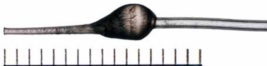
Fig. 1. The tip of cannulation tubing to inject the resin into the digestive organ. One scale=2 mm.
